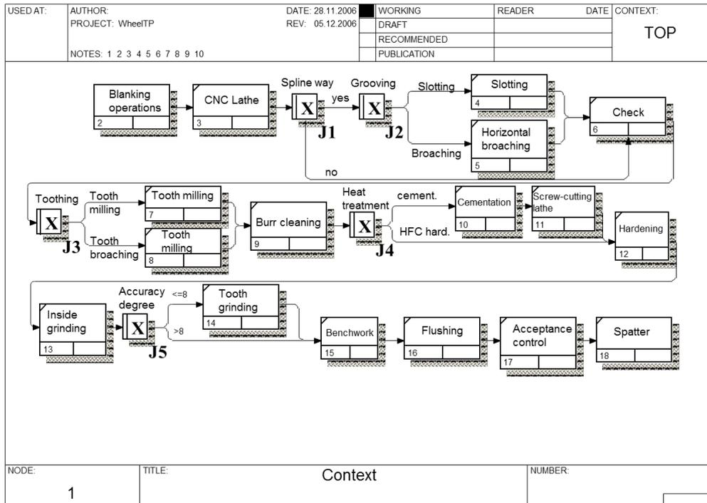
**Fig. 2.** Process Flow Diagram (PFDD) of cylindrical gears
