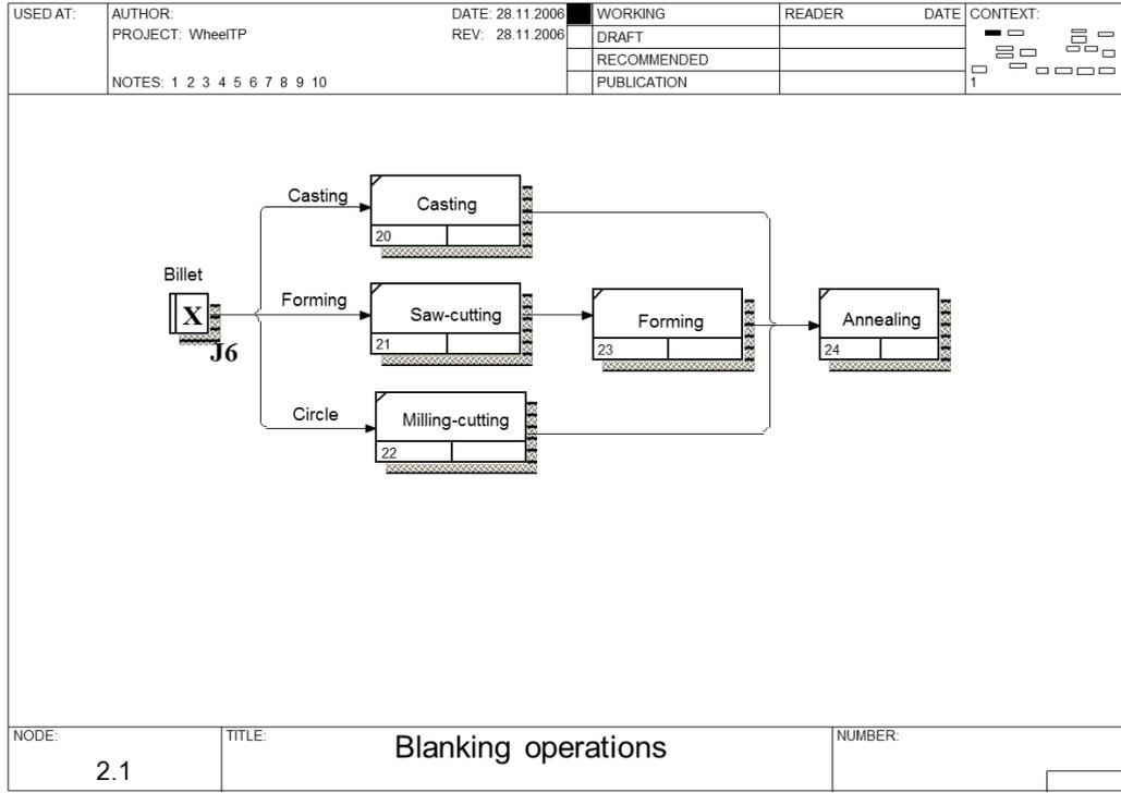
**Fig. 3.** Secondary diagram of blanking operations for cylindrical toothed gears
